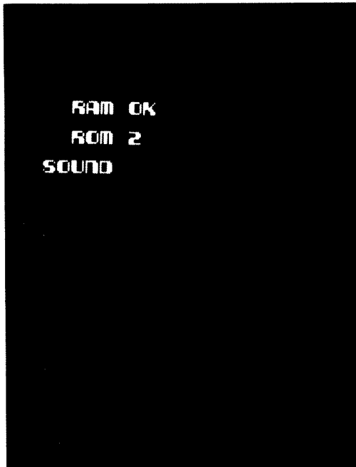
Figure 2-3 Self-Test Display (ROM Failure)
