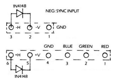
CURE 3: Join negative sync inputs J2 and J3 together with a jumper. Locate WI02 and install a jumper from W102 to either J2 or J3.
