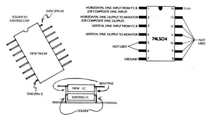
CURE 2: Used for Wells-Gardner Video Sync boards with positive sync connections only. (Vertical mount board 85x140B.
