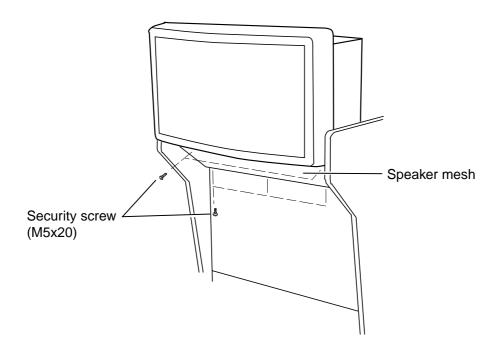
3. Remove 4off pozi head wood screws and remove the left speaker only sufficiently to access the speaker connections.
