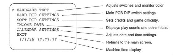
3. Hardware test (If software is not loaded, only the HARDWARE TEST mode can be used.)
