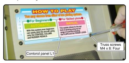
5 After removing the control panel L1, you will find the monitor adjustment panel inside. Adjust the image size while looking at the crosshatch on the screen and adjust the color while looking at the color bar on the screen.
