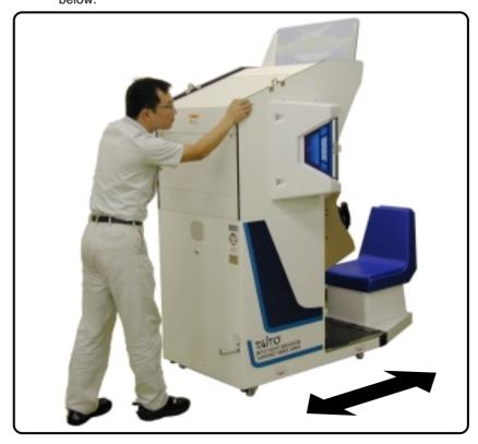
Load the machine on a truck and secure it by lowering the six adjustable feet. Lower the adjustable feet until the casters are raised approximately 3 mm above the truck using a monkey wrench or the like.
