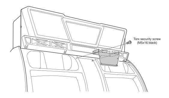
2. Fit the new Vac-Form with 4off Torx security screw (M5x16 black), supplied.
