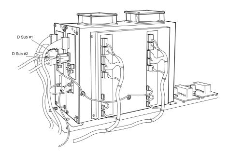
Note: When refitting the D Sub connectors to the Front Boards ensure that connector 2 is fitted to the board nearest the rear of the cabinet, and the connector retaining screws are fully tightened.
