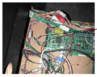
WIRES CONNECTED WITH CRIMPS
