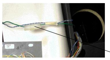
PULL UNTIL THIS CONNECTOR APPEARS. (NOTE: BLUE WIRE TO BE ATTACHED IN STEP 4)
