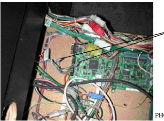
WIRES CONNECTED WITH CRIMPS
