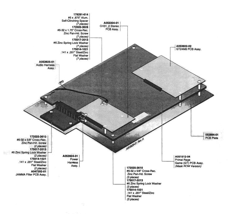
Figure 4-2 Board Stack Assembly (corrected)
