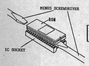
As shown by a drawing, separate them by inserting minus screwdriver alternately not to damage pins.
