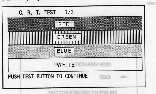
Red, green, and blue are darkest on the leftmost scale and get brighter by 31 gradations to the right. The contrast of the monitor is normal, if the white color bar is black in the leftmost position and is white in the rightmost position.
