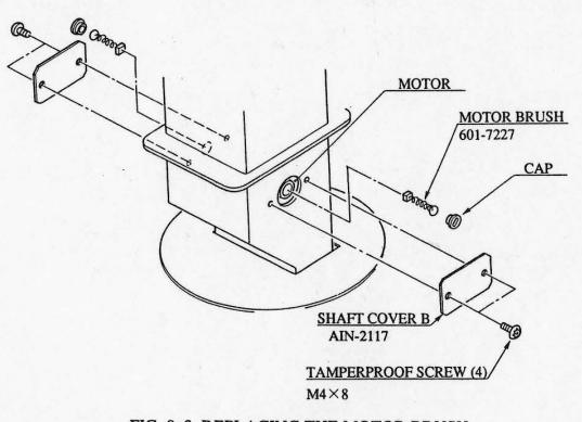
FIG. 9.3 REPLACING THE MOTOR BRUSH
