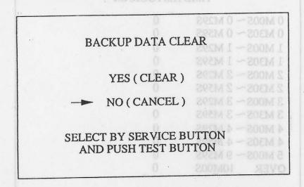
When clearing, bring " $\rightarrow$ " to "YES" and when not clearing, to "NO", by using the SERVICE BUTTON, and then push the TEST BUTTON.
