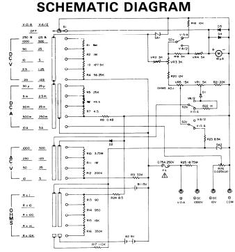
**NOTES:** (1) ALL RESISTANCE VALUES ARE INDICATED IN "OHM" (K =  $10^{\circ}$ OHM, M =  $10^{\circ}$ OHM) (2) ALL CAPACITANCE VALUES ARE INDICATED IN '' $\mu$ F'' (P = 10  $^{-6}\mu$ F)
