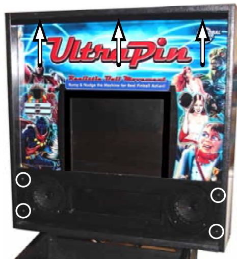
Figure 9. Removing the Backglass Marquee and Speaker Panel
