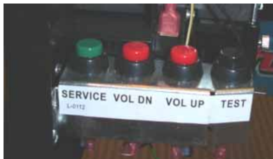
Figure 7. Operator Button Panel
