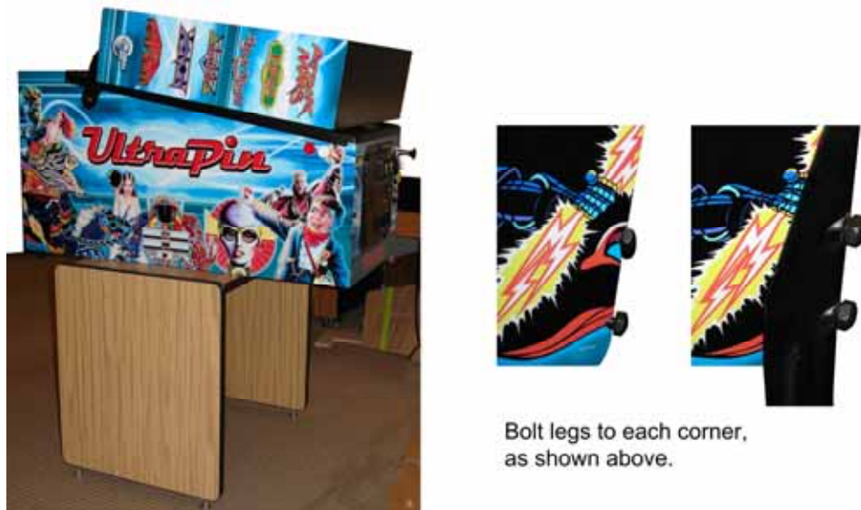
Figure 2. Installing the Legs
