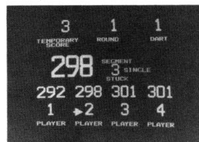
Figure 2. Stuck segment indicator display
