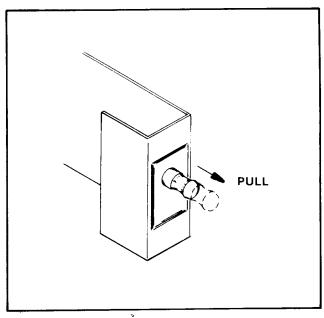
Figure 2-2 Interlock Switch Operation
