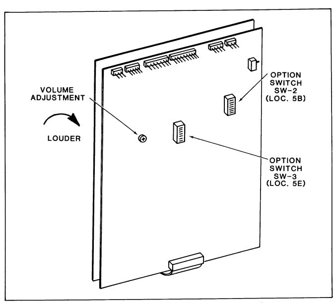
Figure 2-3 Game Volume Adjustment Control & Option Switch Location
